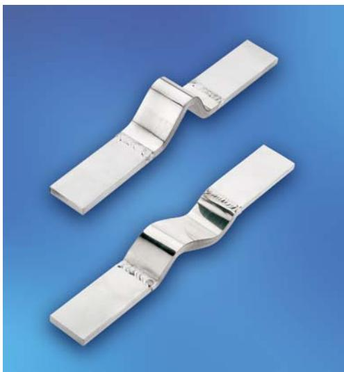
The laminates of our standard aluminium expansion connectors consist out of pure aluminium foils with a thick-ness of 0,3 mm. As contact areas we use solid aluminium pieces. They are welded by an electrical arc and shielded with inert gas to prevent oxidation of the molten bath.
