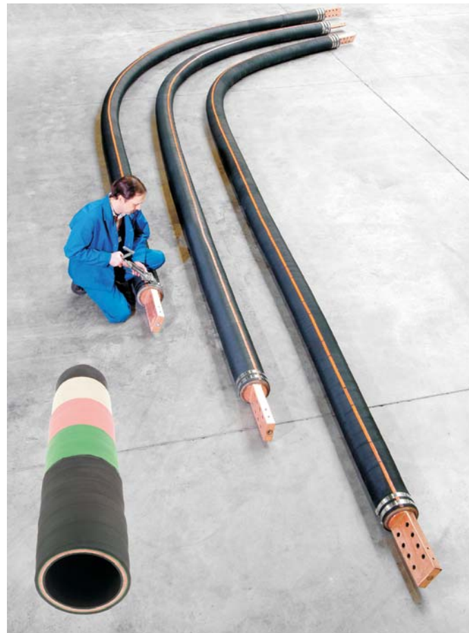
Special coolant water hose with traffic light effect as early warning system
